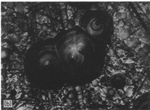
Figure 3 (a) Etch pits produced on the (111) surface of GaAs by the sodium hypochlorite etchant ( \times 60 ). (b) As (a) but ( \times 200 ). (c) Distorted etch pits produced by nitric acid on the (111) surface of GaAs in the presence of some wax.
